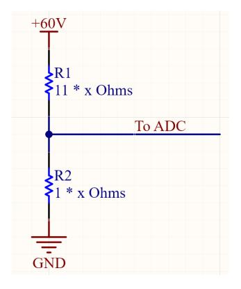
3. The schematic shows a voltage divider. Since no value for the resistance was given in the question, we will assume  $1 \Omega$  for  $R_2$  and use the formula  $R_2 = \frac{U_2}{U}(R_1 + R_2)$  from the lecture where U = 60 Volt and  $U_2 = 5$  Volt. This resolves to  $R_1 = 11$  Ohms.
